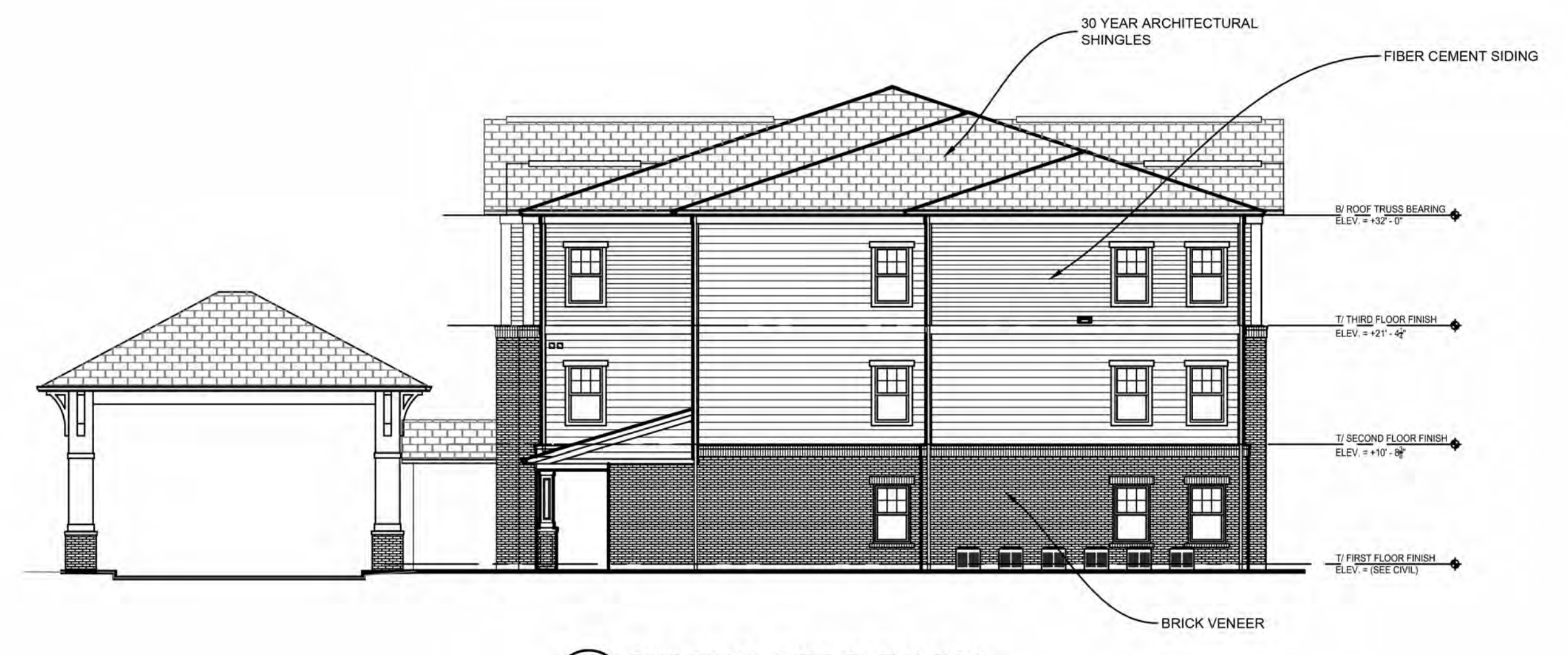
2 BUILDING - SIDE ELEVATION 3/32" = 1'-0"
